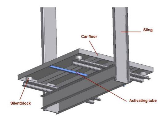
As may be noted, the activating tube links opposite sides of the car floor, and is integrally attached to them, passing through the geometrical centre of the
