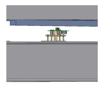
All the above-mentioned is a guideline. Each manufacturer may opt for another solution if it is considered better or more operative. Whatever the option selected is, it is essential that the element that must carry out the activating function does not bend, as, in such a case, measurements would be completely distorted.
