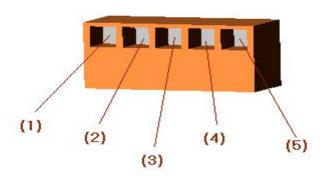
Where connections are as follows, (1) and (2) are feeding connections and (3), (4), (5) are relay outputs.
